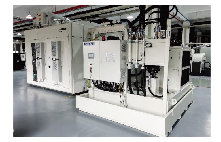
齿轮磨削集中过滤现场 Centralized filtering system for gear grinding machine
