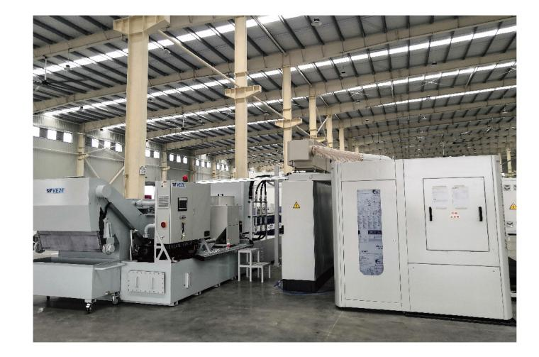
转子(球墨铸铁)磨削专用过滤系统 Specialized Rotor(Ductile Iron) Grinding Filtration System
